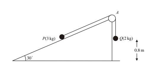
The diagram above shows two particles P and Q, of mass 3 kg and 2 kg respectively, connected by a light inextensible string. Initially P is held at rest on a fixed smooth plane inclined at 30° to the horizontal. The string passes over a small smooth light pulley A fixed at the top of the plane. The part of the string from P to A is parallel to a line of greatest slope of the plane. The particle Q hangs freely below A. The system is released from rest with the string taut.
