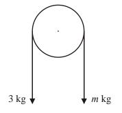
The particles have mass 3 kg and *m* kg, where m < 3. They are attached to the ends of a light inextensible string. The string passes over a smooth fixed pulley. The particles are held in position with the string taut and the hanging parts of the string vertical, as shown in the diagram above. The particles are then released from rest. The initial acceleration of each particle has magnitude  $\frac{3}{7}g$ . Find
