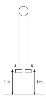
Two particles A and B have mass 0.4 kg and 0.3 kg respectively. The particles are attached to the ends of a light inextensible string. The string passes over a small smooth pulley which is fixed above a horizontal floor. Both particles are held, with the string taut, at a height of 1m above the floor, as shown in the diagram above. The particles are released from rest and in the subsequent motion B does not reach the pulley.
