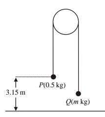
Two particles *P* and *Q* have mass 0.5 kg and *m* kg respectively, where m < 0.5. The particles are connected by a light inextensible string which passes over a smooth, fixed pulley. Initially *P* is 3.15 m above horizontal ground. The particles are released from rest with the string taut and the hanging parts of the string vertical, as shown in the diagram above. After *P* has been descending for 1.5 s, it strikes the ground. Particle *P* reaches the ground before *Q* has reached the pulley.
